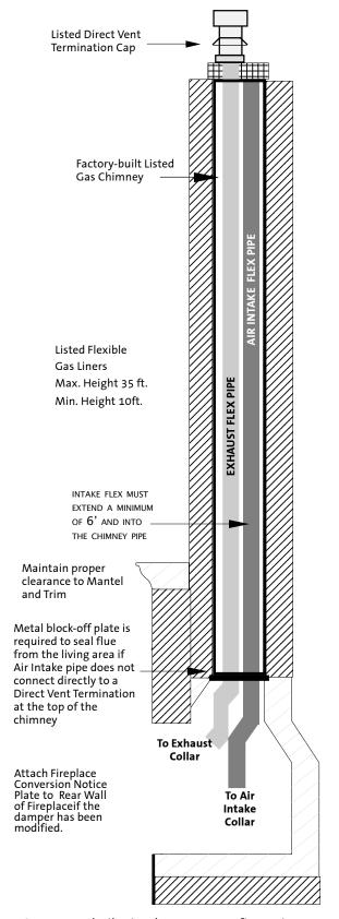
Figure 8. Factory-built Fireplace Vent Configuration.
